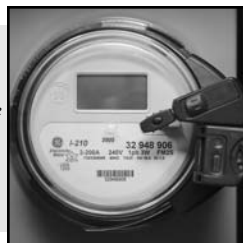
Electronic Meter Measure the distance between the FRONT optical port and the outer rim of the dome. It should be NO LESS THAN 1.5 inches (37 mm). Use Quick Install Guide or see section 5.3
